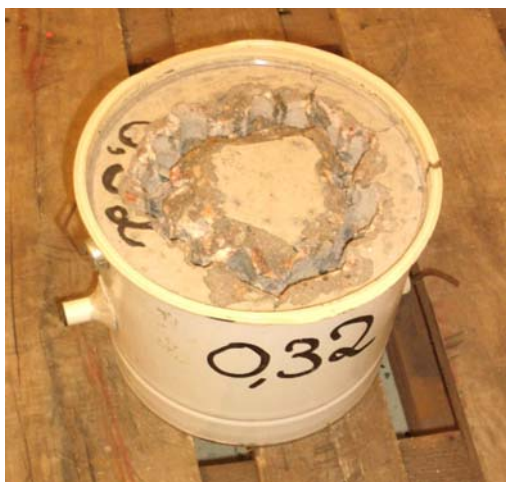
Figur 9. Start uttaget prov vct 0,32.
